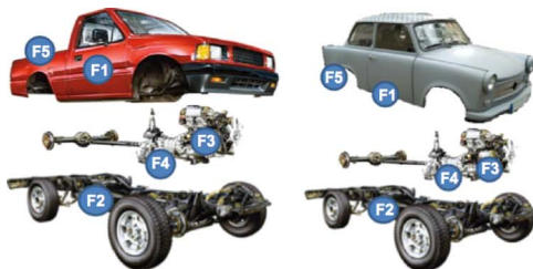
Fig. 4 A schematic of the vehicle architecture design example
