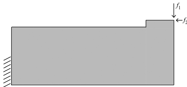
Fig. 9 Design domain for the novel electrical contact
