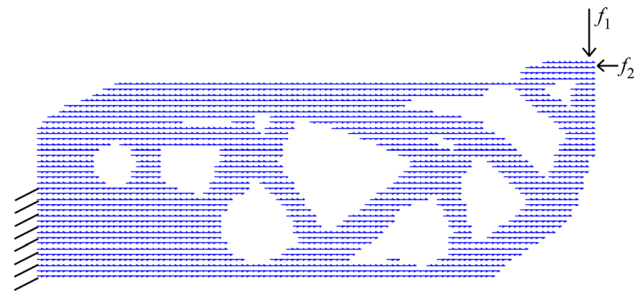
Fig. 11 Case 2: Uniformly oriented topology with 4 forced voids that have been optimally located and sized. C_C = 109.5 and K_C = 192 .
