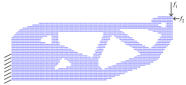
Fig. 10 Case 1:(Benchmark C) Uniformly oriented Topology with no forced voids. C_C = 100 and K_C = 100 .
