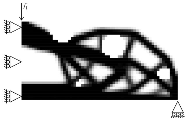
Fig. 7 Resulting topology from using four voids and allowing them to move their location and size to find an optimum solution. C_A = 134 and K_A = 192 .
