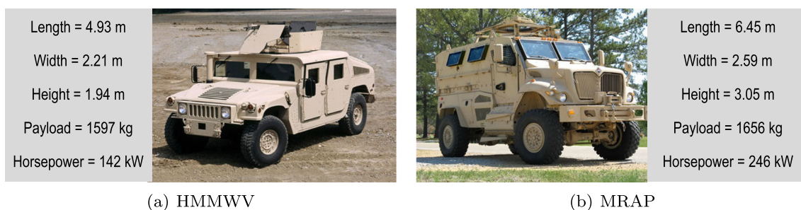
Fig. 6 Two current military ground vehicle options and their associated capabilities (from www.amgeneral.com , www.defense-update.com , www.militaryfactory.com , www.navistardefense.com )
